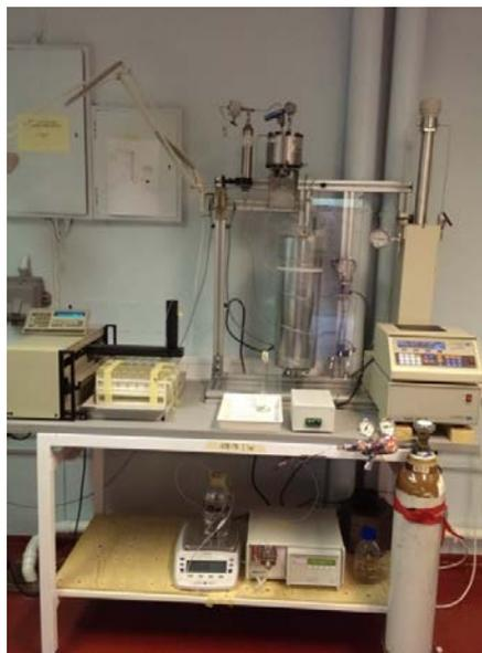
Figure 6 Experimental setup at IFE for monitoring flow of tracer at supercritical conditions.
