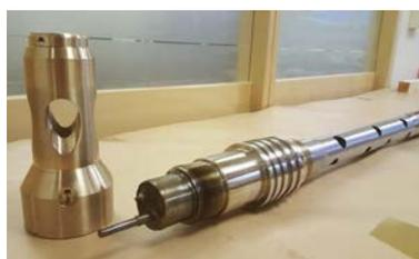
Figure 4 Bulkhead with temperature probe and pressure port constructed for the DESCRAMBLE project
