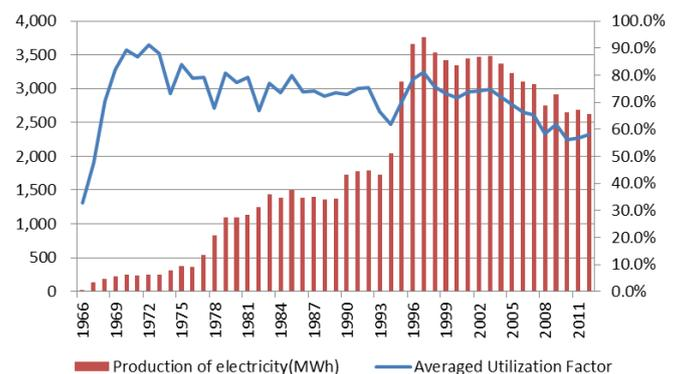
**Figure 3.** Total production of electricity and average utilization factor of geothermal power plants in Japan.
