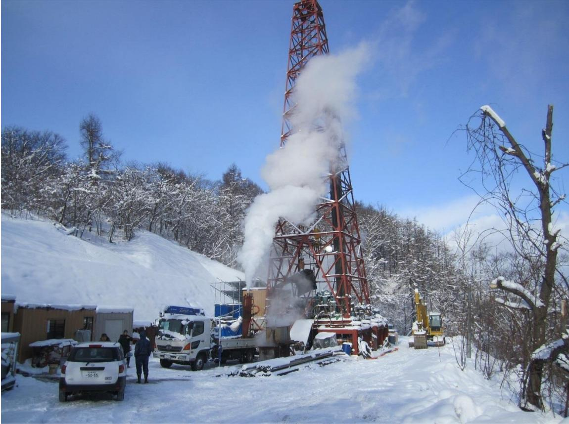
**Figure 1.** Drilling of an investigation well at the Toyako-Onsen field in Hokkaido, Japan, conducted by Toyako Spa Association.
