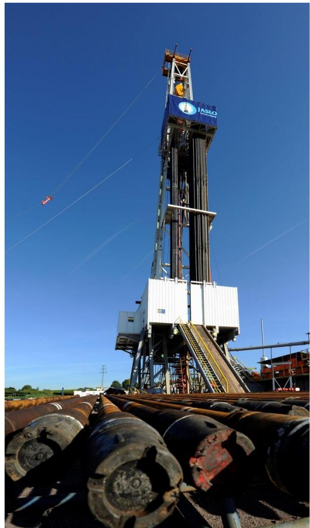
**Figure 4** Geothermal drilling rig at Insheim.
