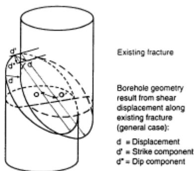
Fig. 7. Determination of slip amplitude from borehole geometry monitoring [9].
