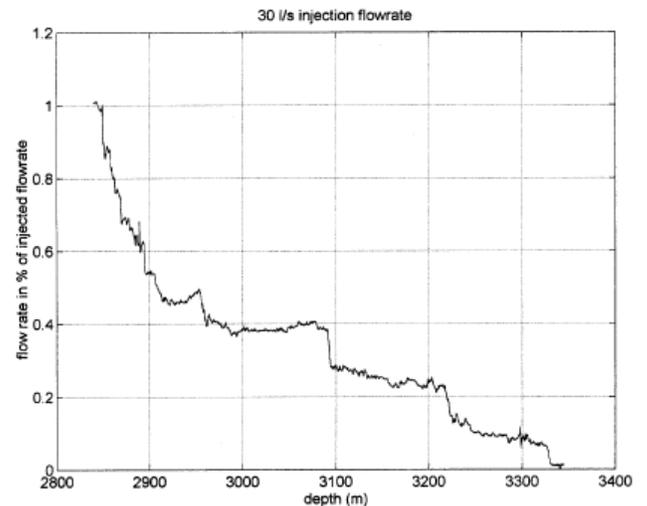
Fig. 3 Flow rate (spinner) log run in GPK1 during the 1993 stimulation. Horizontal axis is depth, vertical axis is percentage of total flow injected in the well (here  $30 \cdot 10^{-3} \text{ m}^3/\text{s}$ ) [11].
