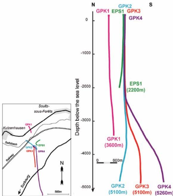
Fig. 2. Geometry of the various wells at Soultz
