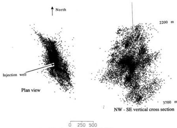
Fig. 4 Horizontal (left) and vertical (right) projections of microseismic events detected with the downhole network. The vertical projection is orientated N 150°E, i.e. parallel to the direction of the maximum horizontal extension of the cloud.
