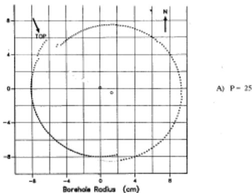
Fig. 6. Determination of the center of a cross section of the well from consecutive ultrasonic shots [9].
