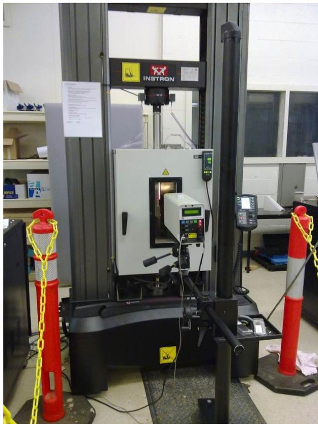
Fig. 4. Servo-controlled Instron machine with a loading capacity of 10 tonnes and environmental furnace
