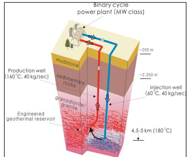
**Figure 15.3** Conceptual model of Korean EGS pilot plant project.
