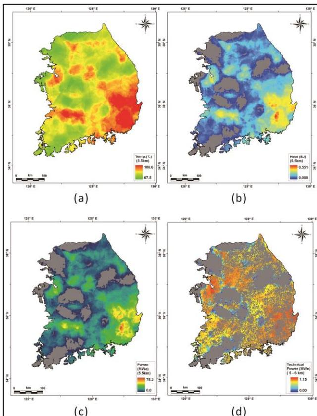
**Figure 15.5** Example of EGS potential assessment procedure: (a) temperature distribution at 5.5 km depth; (b) heat contents in depth range 5-6 km; (c) theoretical potential in depth range 5-6 km; (d) technical potential in depth range 5-6 km. Note that grey regions in (c) and (d) represent area of temperature lower than surface temperature+80 °C, while in (d) include in-accessible area as well.
