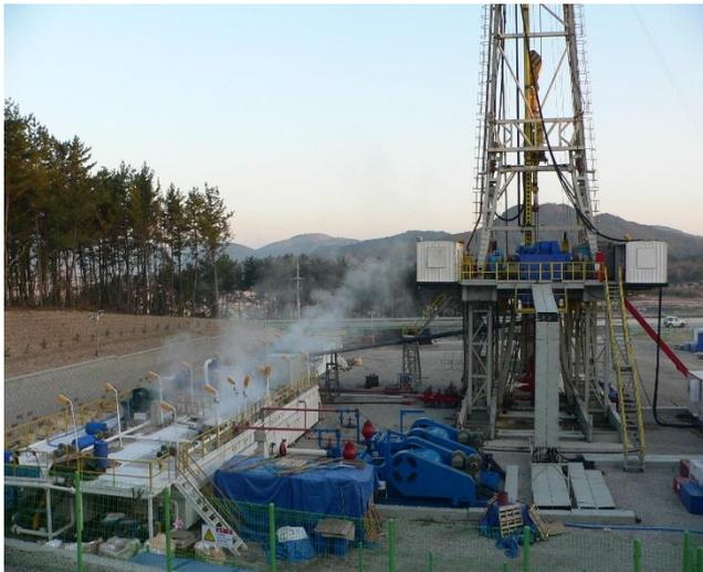
**Figure 15.4** Steam over mud tank as mud was heated by deep circulation during drilling of PX-1.
