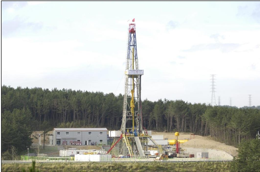
**Figure 15.1** Drill rig with API static hook load of 3,150 kN at the EGS pilot plant project site in Pohang, southeastern part of Korea.
